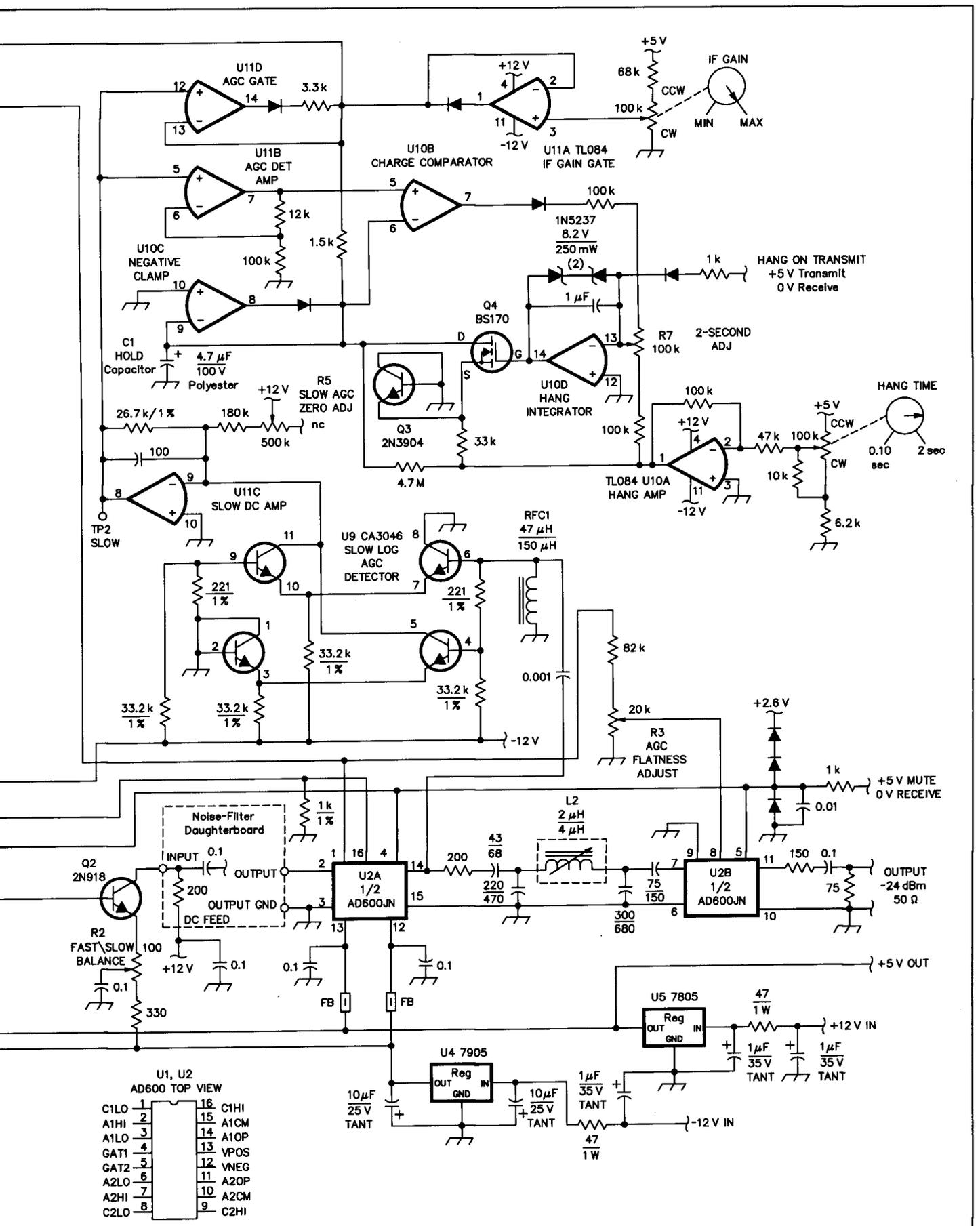
resistor. The resistor value is optimized for the lowest AD600 noise figure. To produce a precise 50- $\Omega$  input resistance, Q1's source current is adjustable and a capacitor across the input terminals cancels the leakage reactance of the feedback transformer, T1. Minimum transformer loss is necessary to achieve a low noise figure, so the input transformer (T1) *must* be wound exactly as shown on a BN-61-202 balun core.
